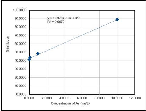
Fig. 2: Linear range and calibration curve for spectrophotometric determination of As  $^{3+}$  based on the inhibition of *G. max* urease activity
