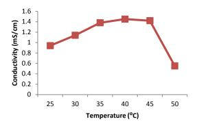
Fig. 3: Effect of temperature on conductometric urease assay
