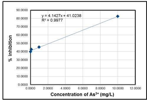
Fig. 1: Linear range and calibration curve for conductometric determination of As <sup>3+</sup> based on the inhibition of G. max urease activity
