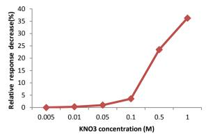
Fig. 5: Effect of ionic strength on conductometric urease assay
